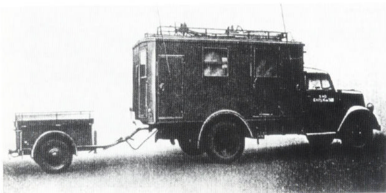
Below: Trough trailer for the Kfz.305/122 decontamination vehicle based on the 1941 Opel Blitz Type 3.6-36 S of the Safety and Emergency Service (S.H.D). (L.Dv.783/5)
