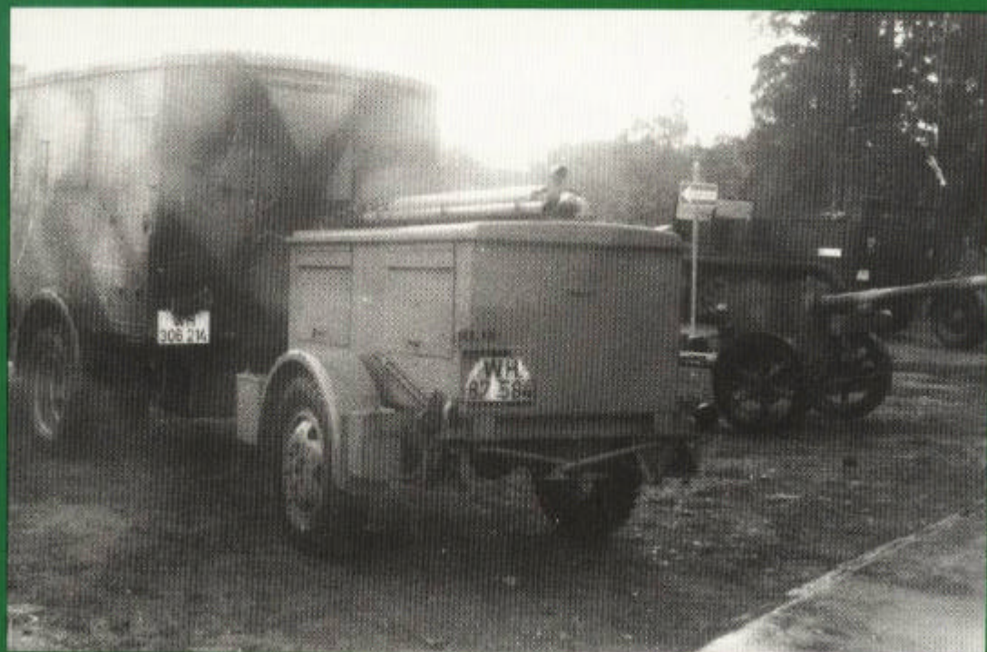
This heavy Type-A field generator unit (SdAh.24) was displayed at the Bundeswehr's Combat Forces School II at Munster on "Armored Fighting Forces Day." The trailer was pulled by a Mercedes-Benz L 3000 S radio truck.
