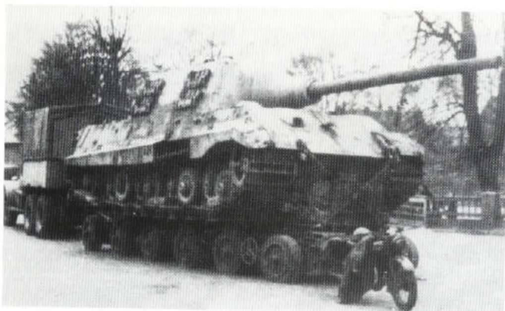
Above: Six-axle trailer by the Gotha Rail Car Factory with a payload of 60 tons, seen here carrying a Jagdtiger (Sd.Kfz.186)
